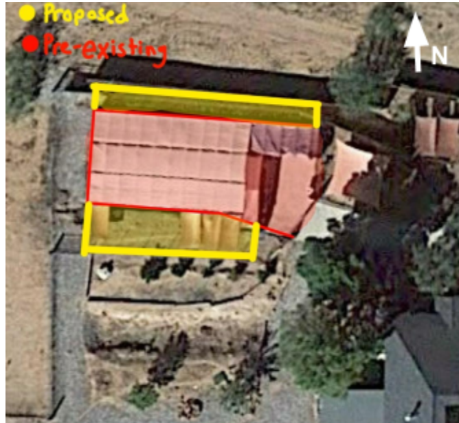
Figure 1-5: A visual of the project site's pre-existing development (red) and the available space (yellow) for the site design.
